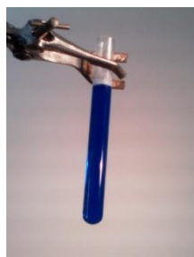
Figure 1: The blue colour of Cu[trientine]^{2+} , obtained by adding a 300 mg trientine dihydrochloride capsule to aqueous copper sulfate.
