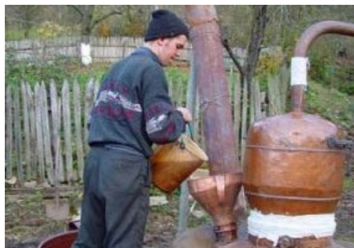
A copper still for distilling tuica
