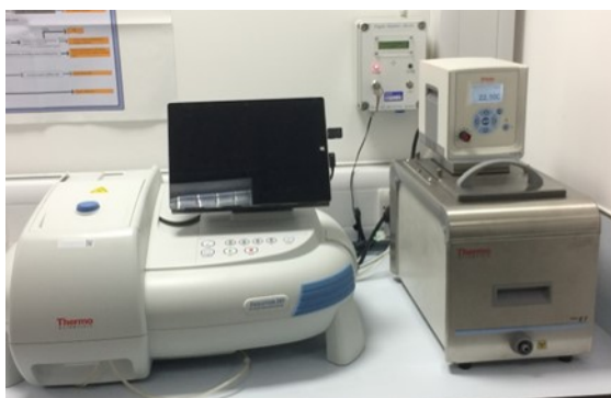
Fig 2. Ultra-violet/visible spectrophotometer used to measure the oxidase activity of the copper containing protein ceruloplasmin.
