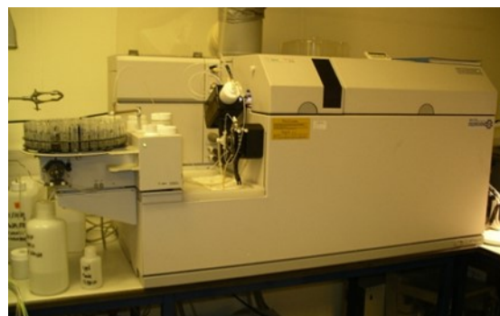
Fig.1. Inductively coupled plasma mass spectrometer for the measurement of copper.
